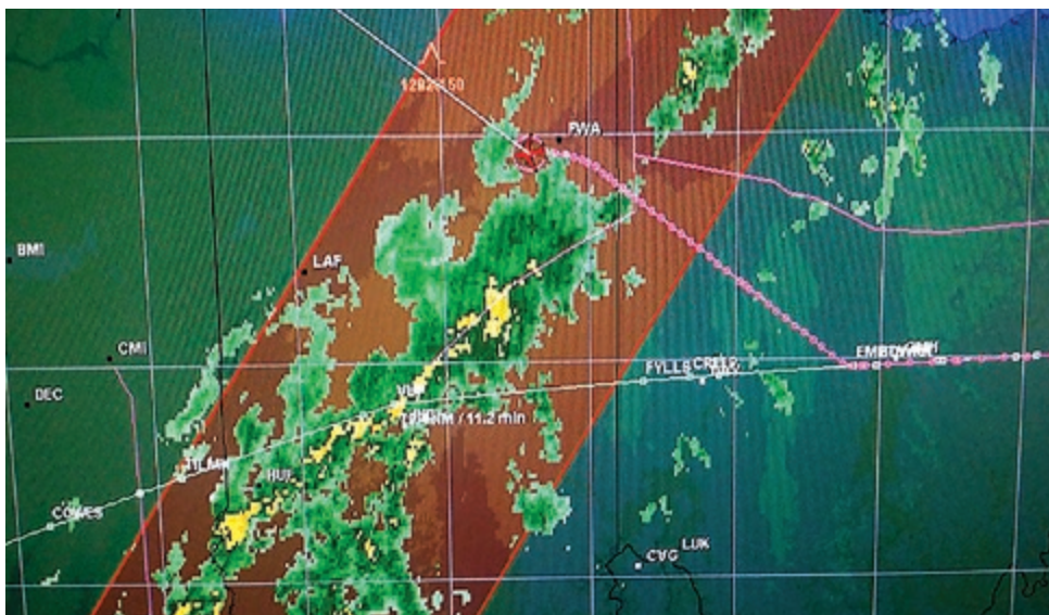
An example of Dispatcher-suggested storm deviation. The green line shows the planned route, and the pink indicates the path actually operated to steer clear of the weather.
